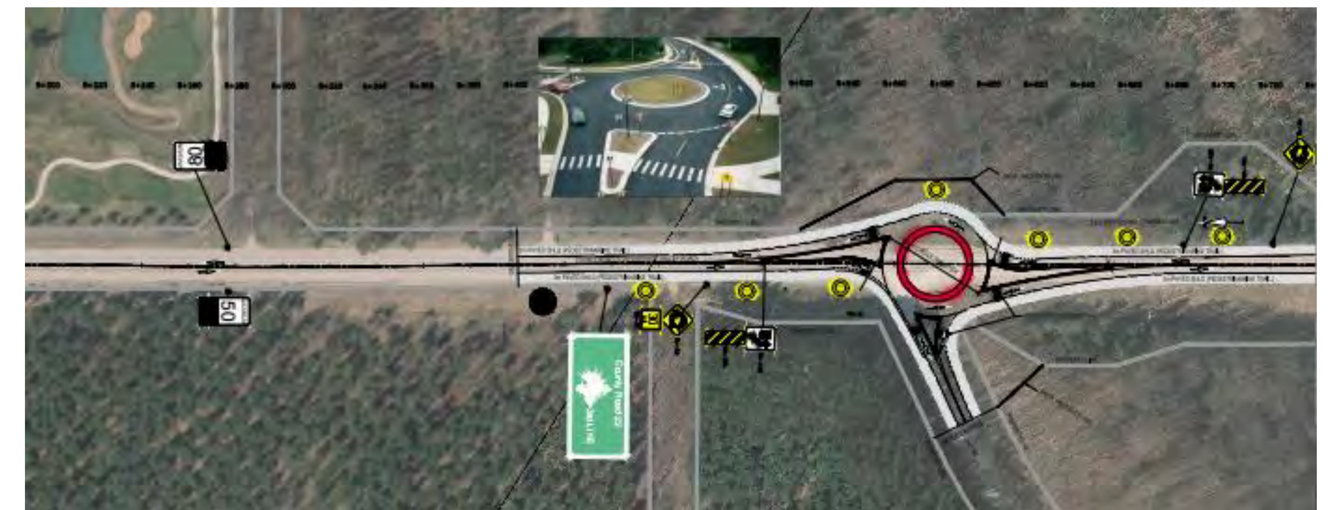
Recommended Intersection Improvements (County Road 22 and Line 3)
