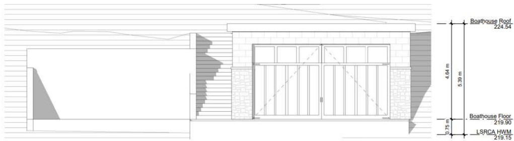
2 Boathouse - South Elevation
