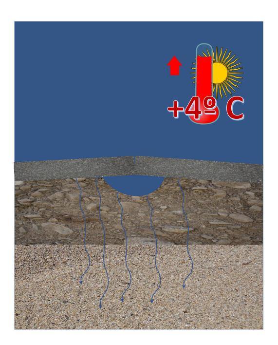
3. When the weather warms up, the ice pockets melt and the water drains through the road base. This not only leaves voids under the roads surfaces but it can also soften the road base.
