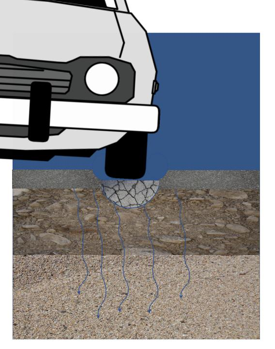
4. The soft, cracked asphalt no longer supports the weight of traffic and breaks up leaving a hole on the surface.
