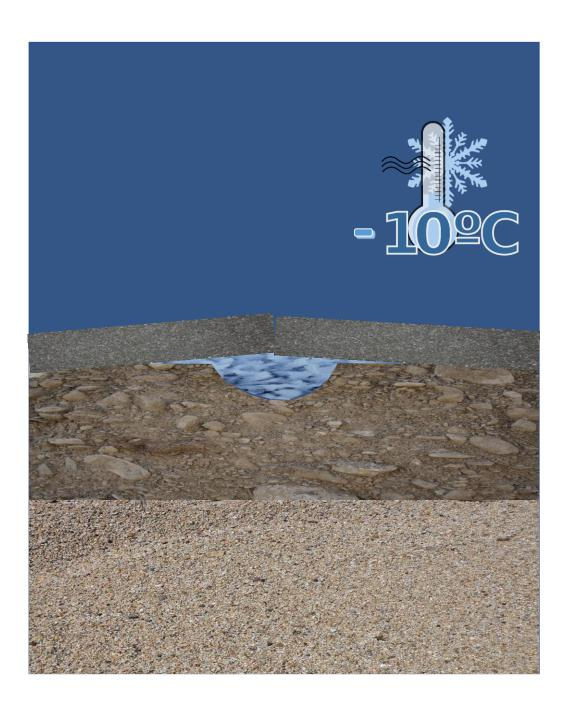
2. Pockets of water form under the road surface. These water pockets will freeze during cold winter weather and are able to support some traffic. The freezing water expands and will make the asphalt heave and crack even further.
