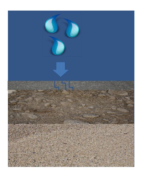
1. Water from rain and melting ice enter the road base through cracks in the surface. The water enters and starts washing away fine particles that hold the gravel base tightly together.
